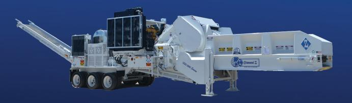
A high-capacity, low-maintenance series essential for any serious grinding application. Features a quick screen change of 20 minutes or less, 1,050 HP, and industry-leading production capabilities.
